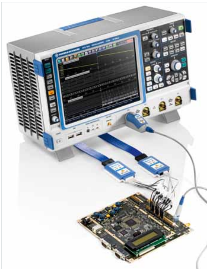
The R&S®RTO-B1 option turns the R&S®RTO oscilloscope into a mixed signal oscilloscope.
