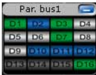
The signal activity of the digital channels is displayed in the signal icon independently of the acquisition state.
